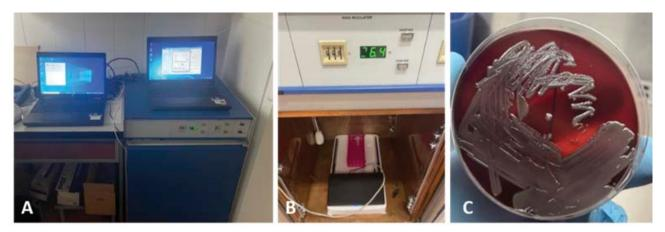
Fig. 2. A- Set of equipment used in the experiment, B- Placement of the exposed sample in the thermostat between the router antennas, C- E. coli cultured on Endoagar
