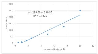
Fig. 1. Standard meloxicam calibration curve (0.5–10  $\mu$ g/mL; R<sup>2</sup>=0.932)
