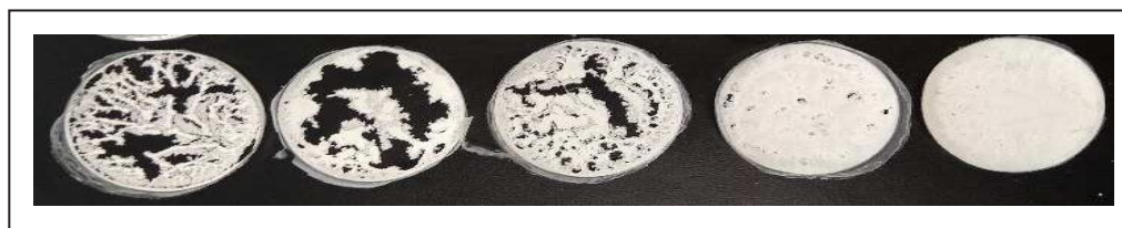
Fig. 2: Patches containing castor oil, dried without a covered funnel
