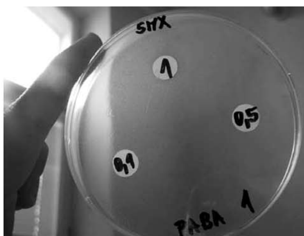
Fig. 1. The visual demonstration of the presence of the inhibition zones formed around the filter paper discs soaked with presented concentrations of sulfamethoxazole standard and their absence after the addition of PABA to the agar medium at the concentration of 1\mu\text{g}\cdot\text{ml}^{-1}
